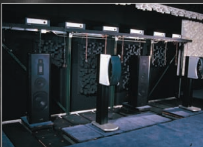
For critical listening, JBL's Speaker Shuffler swaps pairs of speakers in under 3 seconds.
