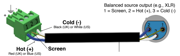
Fig.8 Balanced wiring (US).
