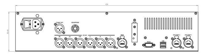
MAINS IEC 320/C14 power inlet (80-240 VAC) with integrated switch
