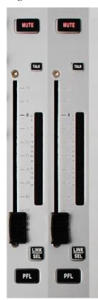
These two channel strips always control the Grand Master faders. These faders are always active, no matter which bay is selected on the touch-screen.
