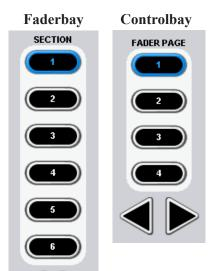
The second level of navigation is the scrolling and banking as it is known from any "real" Vista desk. This is done with the six section buttons and the two arrrows (for the faderbays), respectively with the four fader page buttons and the two arrows (for the controlbay). These section- and fader page buttons can be operated via the touch screen.
