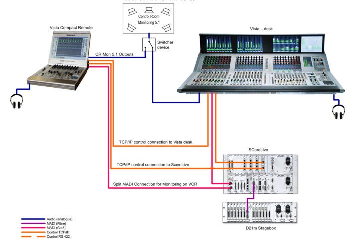
If desk redundancy needs to be achieved with the Compact Remote, it also needs to be connected to the DSP engine, in addition to its network connection to the Vista desk. This way it is capable to continue a mixing session in case of a desk failure.
