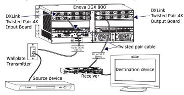
FIG. 1 DXLINK TWISTED PAIR 4K TX AND RX ENDPOINT SOLUTION (CONNECTED TO DGX800-ENC)
