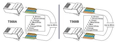
FIG. 3 RJ-45 PINOUTS
