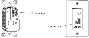
FIG. 5 ATTACH SIGNAL AND TRANSPORT CABLES ON DX-TX-DWP-4K
