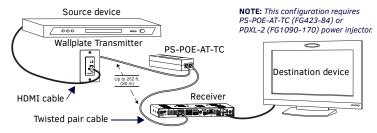
$\textbf{FIG. 2} \ \ \textbf{DXLINK TWISTED PAIR 4K TX AND RX AS EXTENDER SOLUTION}$
