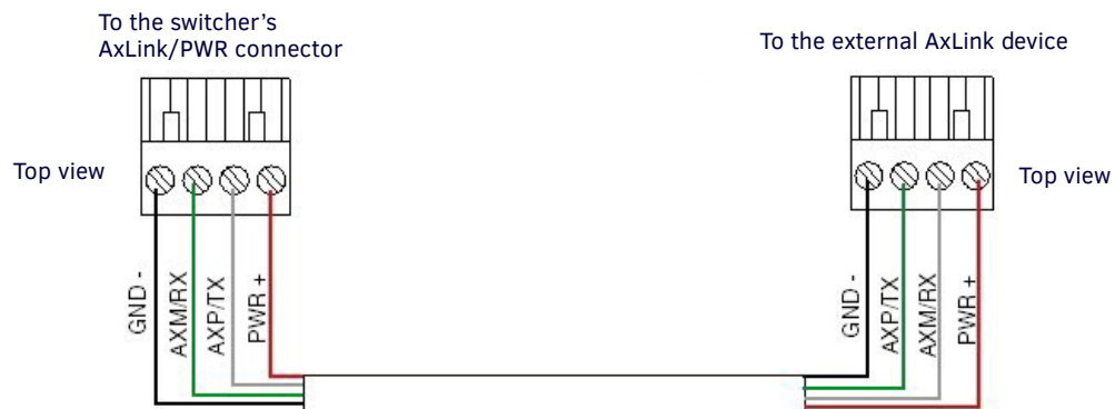
FIG. 27 Mini-Phoenix connector wiring diagram (direct data and power)
