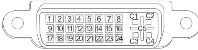
FIG. 21 DVI pinout for DVI-to-HDMI cable adapter
